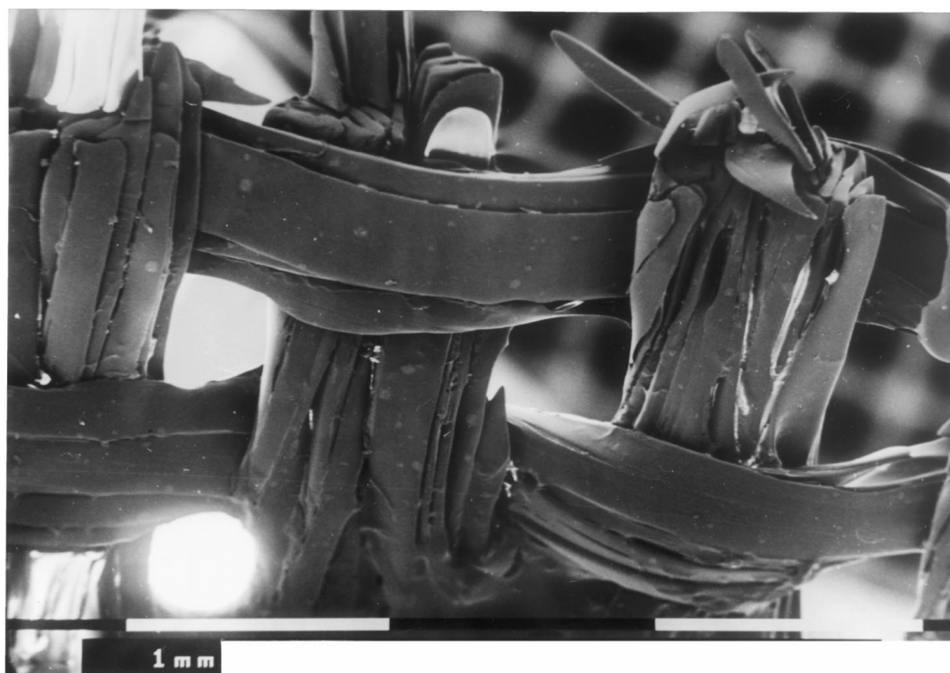
Figure 2 SEM micrograph of the original woven polypropylene fabric.
