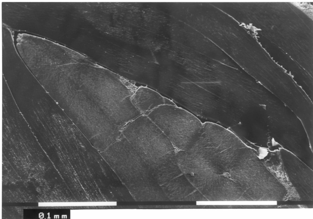
Figure 5 SEM micrograph of an etched sample compacted at 172 °C. Recrystallized material can be observed at a number of locations between adjacent tapes.
